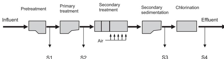
**Fig. 1.** Procedures Used for Sewage Treatment and STP Sampling Points (S1–S4)
