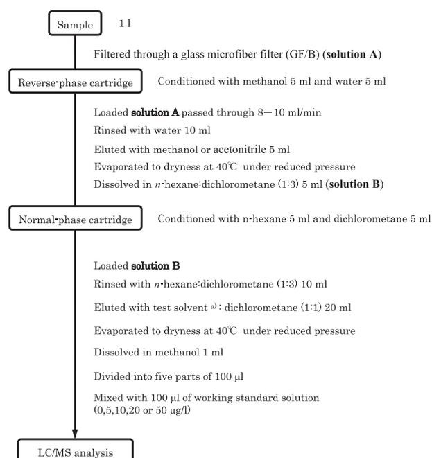
**Fig. 2.** Schematic Representation of the Analytical Method
